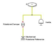
Based on the value you select for the Specify inertia parameterization by parameter, you specify inertia J directly or using the machine inertia constant H.
