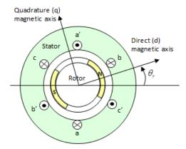
For the axes convention in the preceding figure, the a-phase and permanent magnet fluxes are aligned when rotor angle  $\theta_r$  is zero. The block supports a second rotor-axis definition. For the second definition, the rotor angle is the angle between the a-phase magnetic axis and the rotor q-axis.
